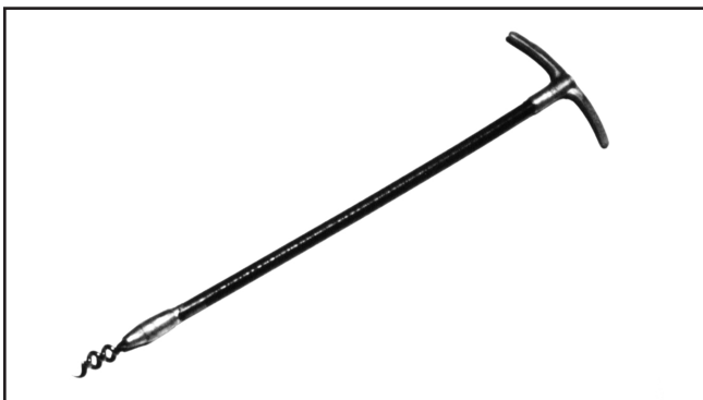
Figure 5.1E Flexible packing removal tool cork screw tip
