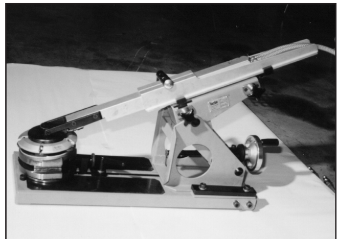
Figure 5.2B Wedge or disc automatic grinding machine
