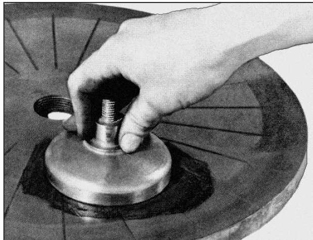
Figure 9.9A Lapping of disc
